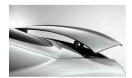
Rear spoiler extendable, manually by a push button or automatically from speeds of 120 km/h
