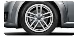
Cast aluminium wheels in 5-twin-spoke star design size 8.5 ] x 17 with 245/45 R 17 tyres<sup>1</sup>
