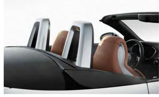
Roll-over bars with trim in aluminium look provide increased safety for driver and front passenger
