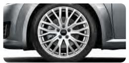
Cast aluminium wheels in 10-V-spoke design partly polished<sup>2</sup>, size 8.5 ] x 18 with 245/40 R 18 tyres<sup>1, 3</sup>
