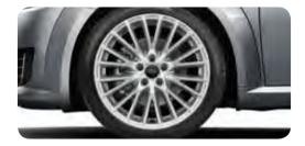
Cast aluminium winter wheels in 20-spoke V-design size 8.5 ] x 18 with 245/40 R 18 tyres<sup>1</sup>, cannot be fitted with snow chains, permissible top speed 240 km/h
