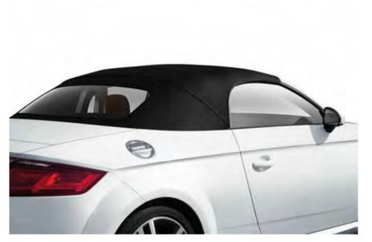
Quality enhanced, exterior noises reduced: the fully automatic acoustic hood made from insulated 3-layer fabric captivates with its high-quality covers in three different colours. It can be opened and closed at speeds of up to 50 km/h in 10 seconds and ensures a pleasantly quiet ride as well as excellent heat insulation.
