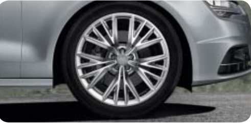
Forged aluminium wheels in 5-spoke W design size 9 J x 20 with 265/35 R 20 tyres 1
