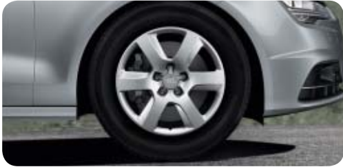
Forged aluminium wheels in 6-arm design size 8 J x 17 with 235/55 R 17 tyres 1
