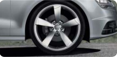
Audi Sport cast aluminium wheels in 5-arm rotor design size 9 J x 21 with 275/30 R 21 tyres 1
