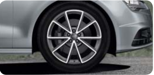
Audi Sport cast aluminium wheels in 5-V-spoke design in matt titanium look, gloss turned finish 2,3 size 9 J x 19 with 255/40 R 19 tyres 1
