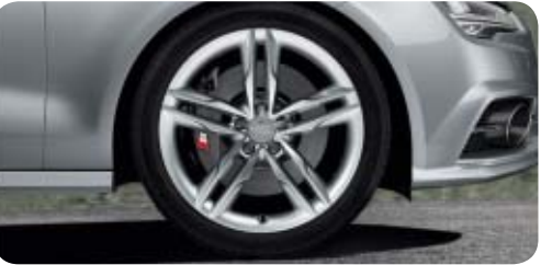
Cast aluminium wheels in 5-parallel-spoke star design (S design) size 9 J x 20 with 265/35 R 20 tyres 1 . Only available for S7 Sportback
