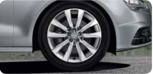
Cast aluminium wheels in 5-V-spoke design size 8.5 J x 19 with 255/40 R 19 tyres 1
