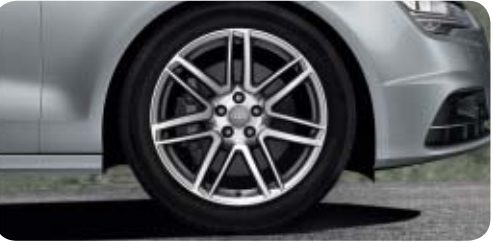
Audi Sport cast aluminium wheels in 7-twin-spoke design 3 size 9 J x 19 with 255/40 R 19 tyres 1
