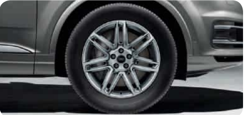
Audi Sport cast aluminium wheels in 7-twin-spoke design with RS logo 3,4 size 8.5 J x 19 with 255/55 R 19 tyres 1
